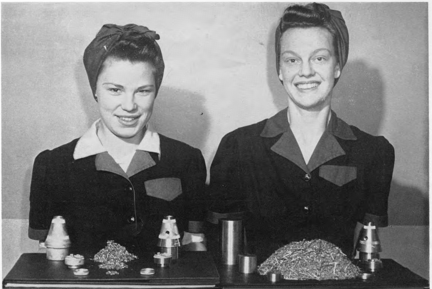
Constantly on the lookout for ways and means of saving critical materials, GM engineers have developed new production techniques which are saving impressive quantities of vital war metals. Illustrated, above, is a noteworthy example of material saving and cost reduction, by the substitution of zinc alloy in place of brass. At the right, Carrie Betts shows the old method of machining down brass bar, while on the left Freda Lindenback displays the new die-cast method which saves fifty million pounds of brass each year.
